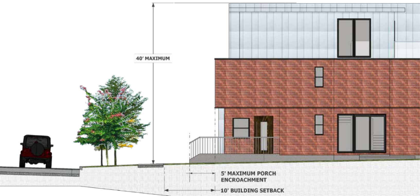
Figure B: Multiplex Building Setback and Height
