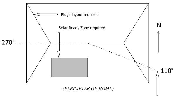
Azimuth is optional. Arrow indicating true North is required.
